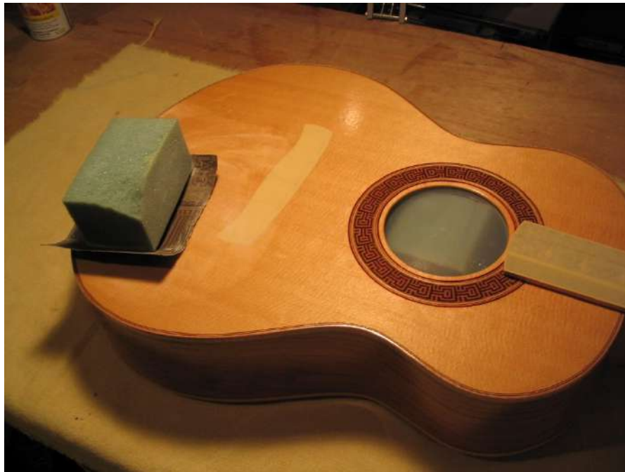
A close-up view of "orange peel", before it is sanded flat.
