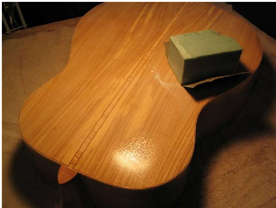
A close-up view of "orange peel", before it is sanded flat.
