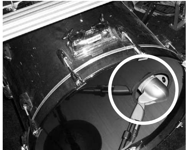
Image 8: Example of bass (kick) drum mic placement
