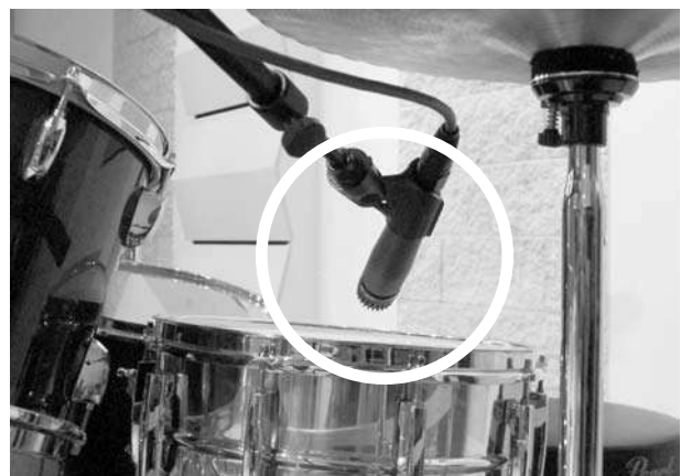
Image 9: Example of snare drum mic placement
