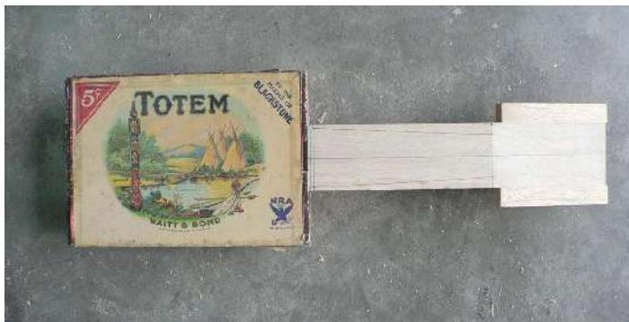
Lay the top on the body, and mark where the Bridge and sound hole will be.
