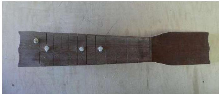
Install the frets into the frets slots. Clip the fret wire to length and press or tap into the slots. Tip: brush a small amount of water into the fret slots to soften the wood fibers before pressing in the frets.
