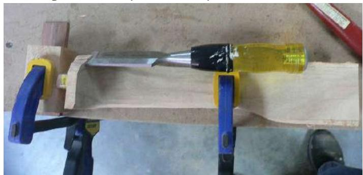
I use chisels for rough shaping, then progress to the belt sander, then hand shaping with flexible shaft
